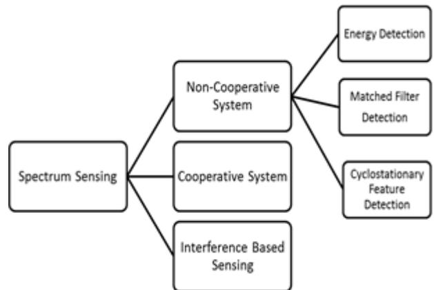
Fig. 2 Classification of Spectrum sensing technique.
