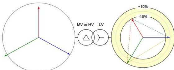
Fig. 1. Voltage imbalance due to unbalance loads.
