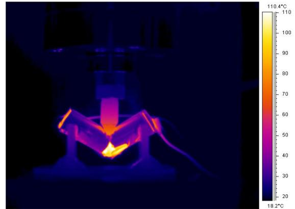
Fig. 4 Thermal hotspot of 3-point bending test
