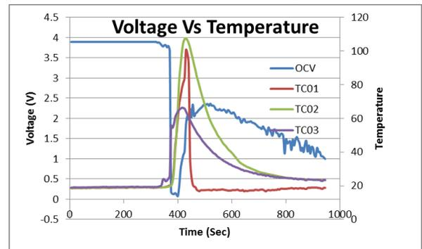
Fig. 6 Voltage and temperature relationship due to Rod indentation test
