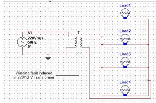
Fig. 2 Winding fault test simulation circuit
