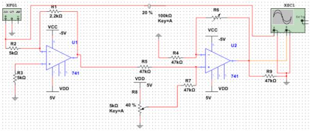
Fig. 3 Signal conditioning simulation circuit
