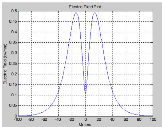
Fig 9: Electric Field Plot 220 KV Tower
