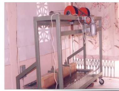
Figure 9: Mobile lift manufactured for Baked Clay Beams
