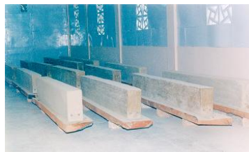
Figure 4: Photographs showing the holes provided for tension & compression bars and at the top for shear reinforcement.
