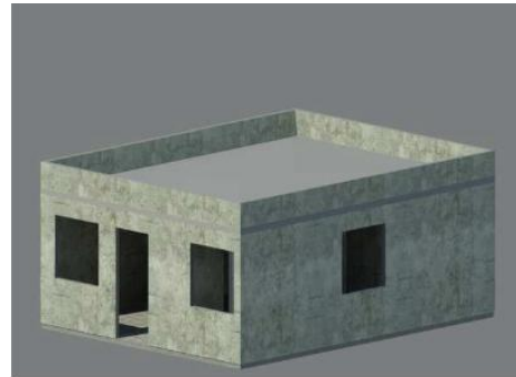
Figure 5 3D-LP walls and roof cover of mortar and concrete
