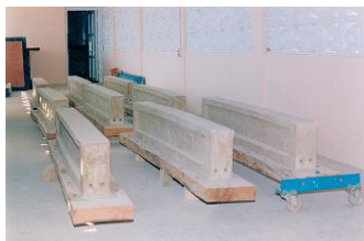
Figure 4: Photographs showing the holes provided for tension & compression bars and at the top for shear reinforcement.
