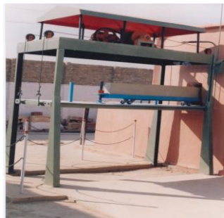
Figure 8: The Photographs showing Platform Lift fabricated for lifting the beam to be placed in the kiln
