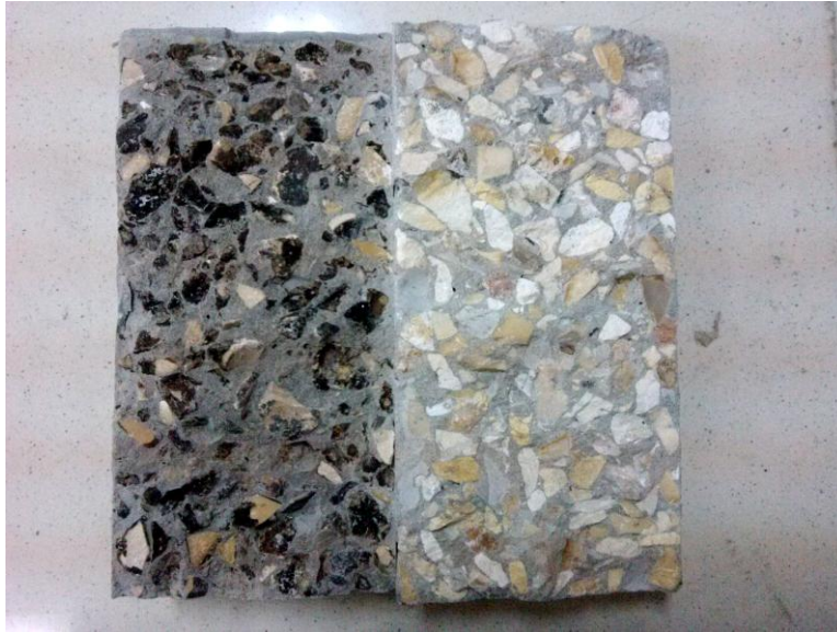
Figure 2: Split cylinder specimens made by dismantled road aggregate and virgin aggregate.
