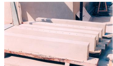
Figure 4: Photographs showing the holes provided for tension & compression bars and at the top for shear reinforcement.
