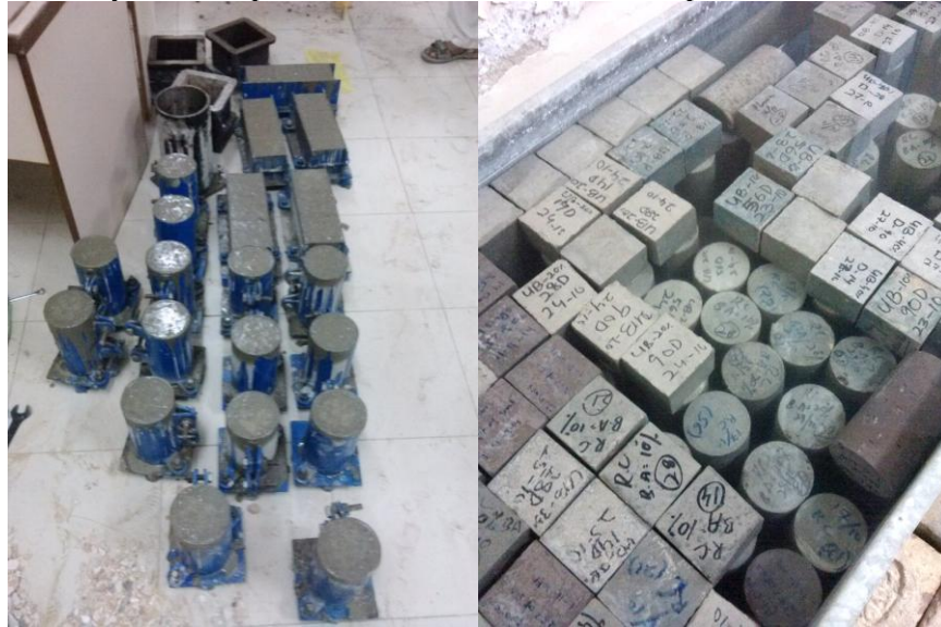
Figure 1: Casting of concrete specimens that are later put in curing tub.
