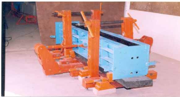
Figure 1: Strengthening of the mould by welding the stiffeners and other strengthening system to avoid the bulging
