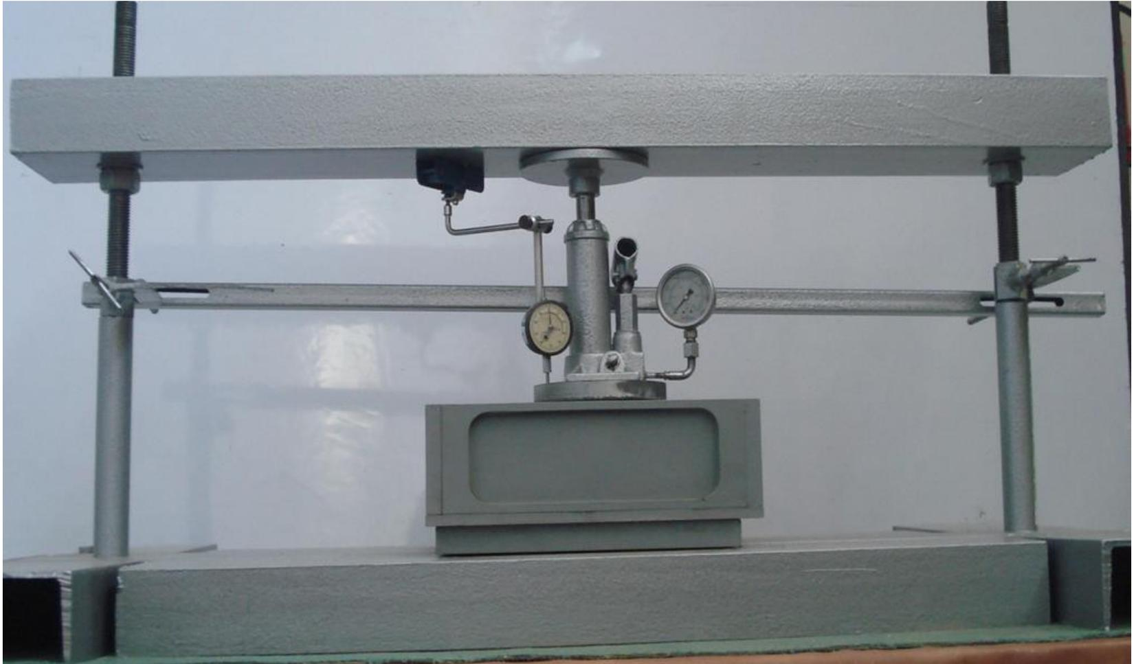
EXPERIMENTAL SETUP FOR REINFORCED SUBGRADE TESTING
