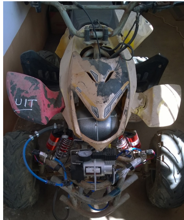
Picture 1 ATV vehicle installed with Electro-Pneumatic Suspension control system.
