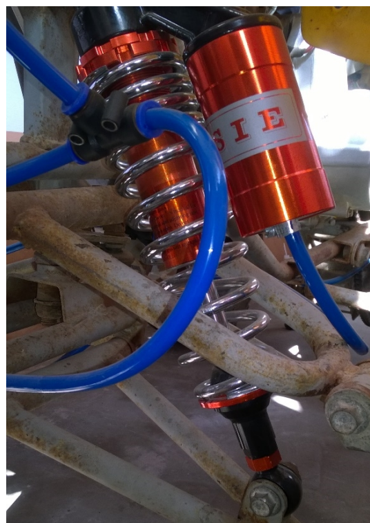
Picture 2 Remote Reservoir Gas Damper installed in the ATV with high pressure air-line connected.
