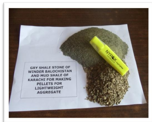
Figure 5. For making pellets, a circular disc type shape using fine and ground grey shale stone of district Lasbella Balochistan with mud shale of Karachi
