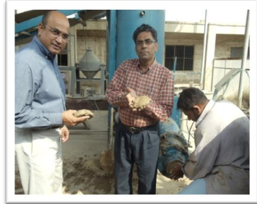
Figure 14. Showing rounded shaped blended pellets are ready for making lightweight aggregate
