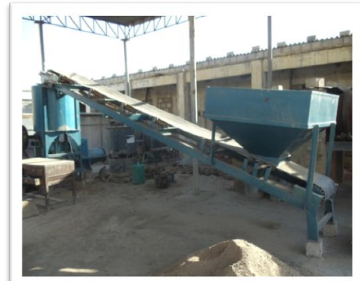
Figure 15. A process of making pellets by pellet mill (semi automatic pelletizer) has been used.
