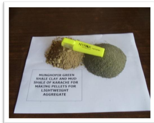
Figure 4. Pellets are made by mixing of fine and ground green shale clay with mud shale of Manghopir Karachi
