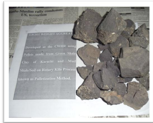
Figure 8. Expanded lightweight aggregate are developed by using green shale clay of Manghopir mixed with fine mud/soil of Karachi
