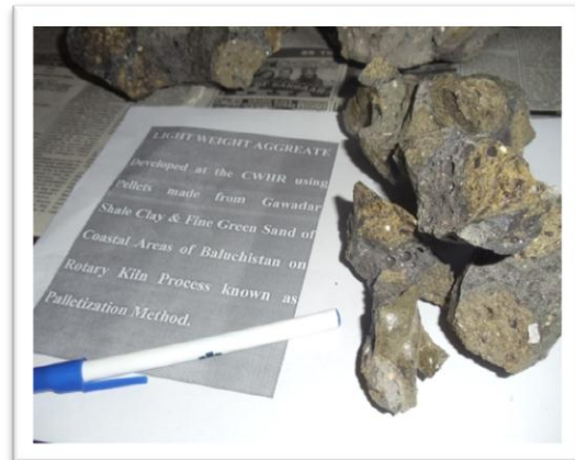
Figure 9. Expanded lightweight aggregate are developed by using Ghuwadar fine and ground grey shale clay mixed with fine dune green sand/ diatomaceous filler
