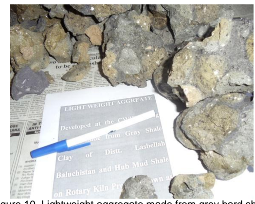
Figure 10. Lightweight aggregate made from grey hard shale of district Lasbella (Winder) shale clay of Karachi
