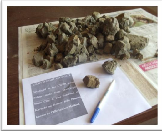
Figure 11. Expanded lightweight aggregate are developed by using Manghopir mud/ shale clay with fine sand of Karachi
