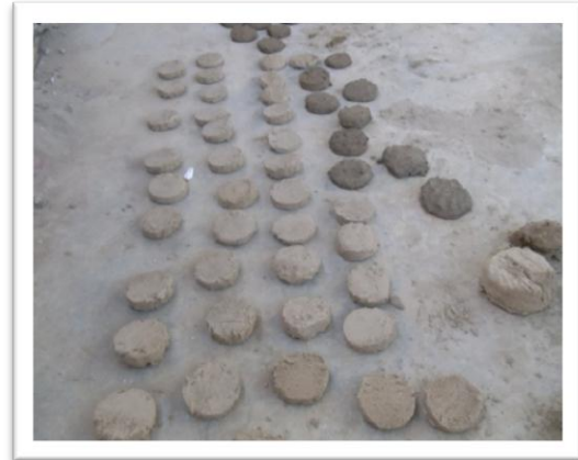
Figure 16. A rounded disc type pellets made from blended mixes of shale clay and fine sand with optimum water requirements
