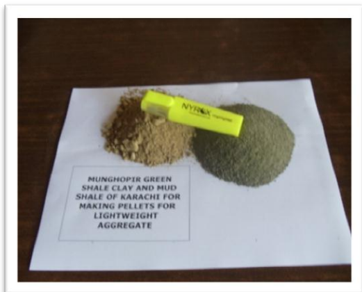
Figure 7. These are Manghopir green shale and mud shale of Karachi used for making pellets of lightweight aggregate
