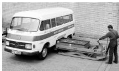
Fig 7. An electric Vehicle charging station replacing batteries with charged ones
